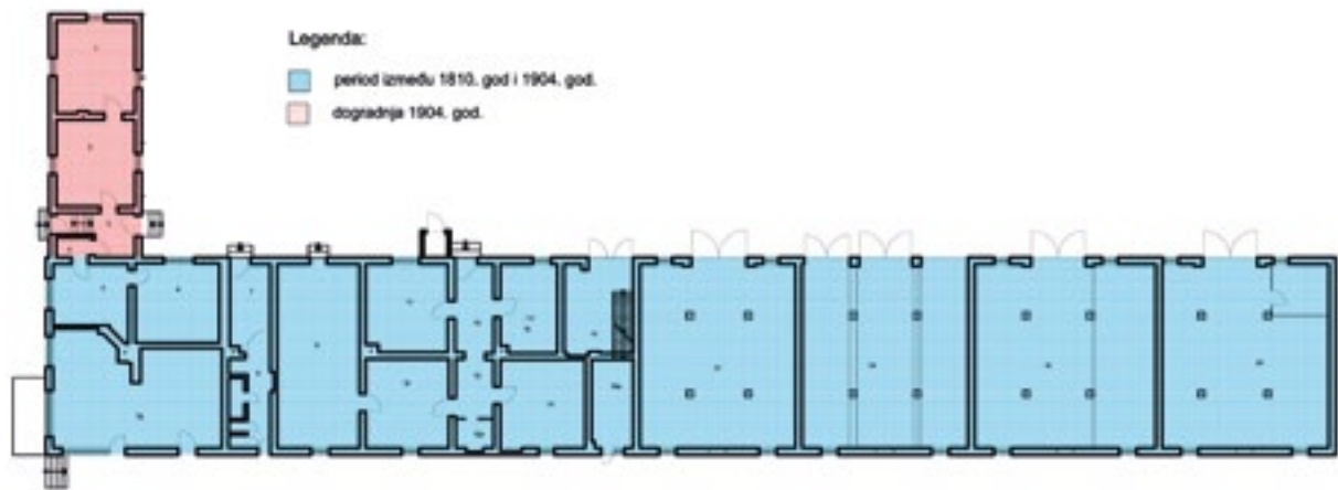
13. Velika Hornwerk vojarna, tlocrt prizemlja, faze izgradnje (dokumentacija HRZ-a, podloge izradio S. Lovrinčević, obradile I. Pauk Sili, V. Giener) Large Hornwerk Barrack, ground-floor plan, construction phases (Croatian Conservation Institute documentation, drawings by S. Lovrinčević, edited by I. Pauk Sili, V. Giener)
